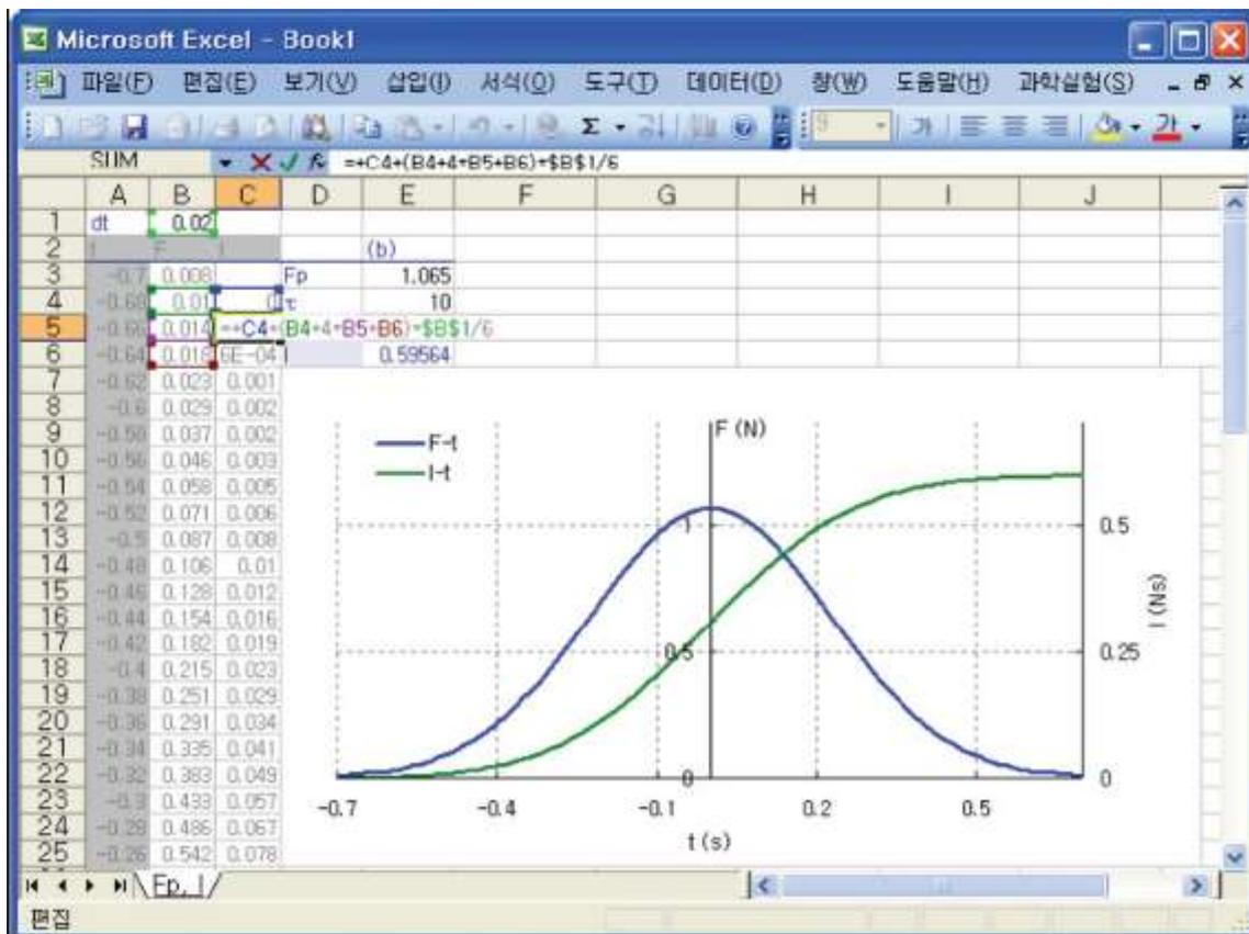
Picture 1.2.4 I-t graph resulted from F-t graph integration: the value of I-t graph corresponds to the value of integration.
